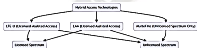
FIGURE 1. Three hybrid access technologies for LTE licensed and unlicensed spectrum (LTE-U, LAA, and MulteFire).
