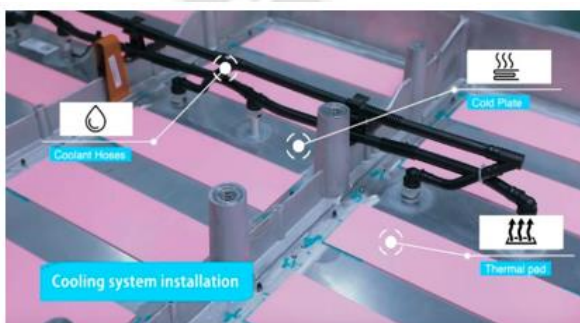
Figure 3. Aerial picture of the vehicle testing battery cooling system
