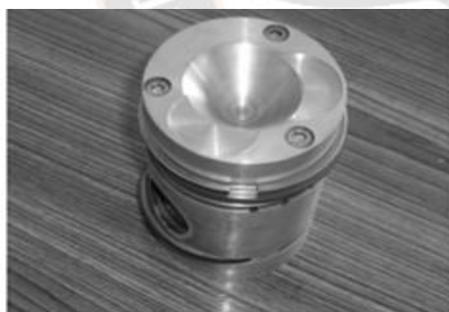
Fig.1 BRASS CROWN PISTON WITH AIR GAP
