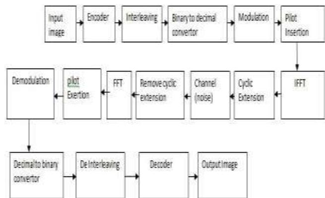
Figure 1: Block Diagram of OFDM Transceiver System
