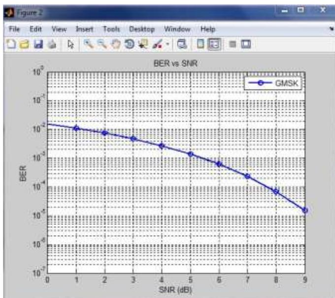
Figure 8: Bit Error Rate Performance of GMSK
